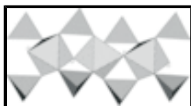
Fig. 3. A polyhedral representation of the one-dimensional Al—O—Al chain of the title compound.
